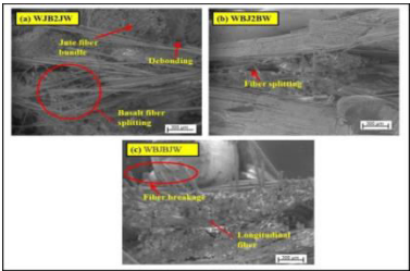
Figure 8 Typical tensile fracture SEM images basalt/jute/ wire mesh composites
